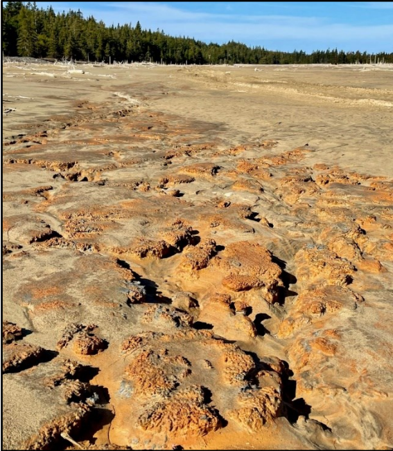
Weathered, sulphide-rich tailings at the abandoned Stirling Zn-Pb-Cu-Au-Ag Mine, Cape Breton, NS (October 2023)
